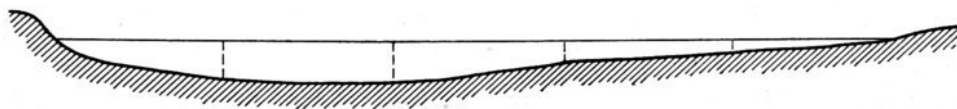
Fig. 45. Left. 2.20 2.71 1.29 0.80 = depth. Right. 72 54 54 59 } velocity. 71 86 69 49 Breadth = 52.00 m. Kuruk-asti, October 2. Scale 1 : 500.
