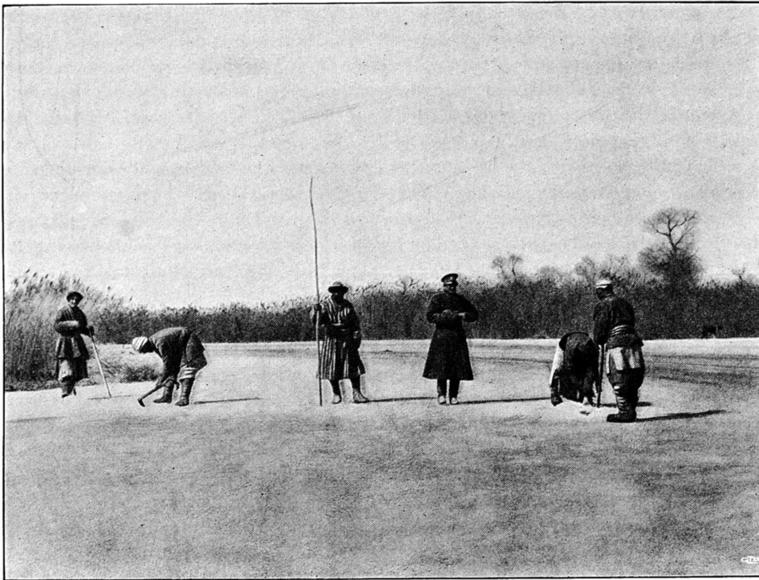
Fig. 7. MEASURING THE KONTSCHE-DARJA THROUGH HOLES IN THE ICE.
