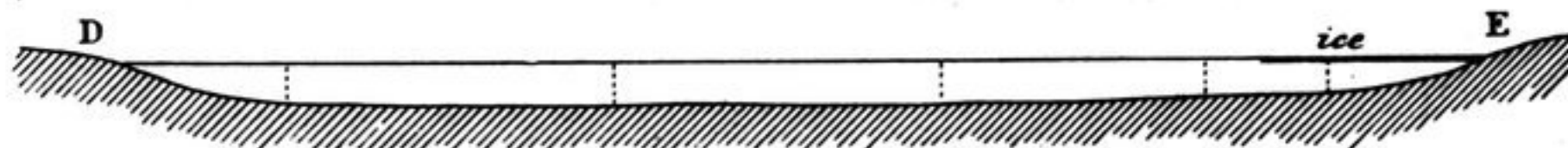
Fig. 220. 29.38 31.76 31.13 26.79 26.30 = depth. Horizontal scale = 1 : 20,000. Vertical scale = 1 : 10,000.
